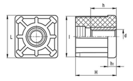
$\begin{array}{lll} d & = M10 \\ h & = 10 \\ H & = 45 \\ h1 & = 10 \\ Internal tube size = 47.0 \\ I & = 47.0 \\ L & = 50 \\ \end{array}$
